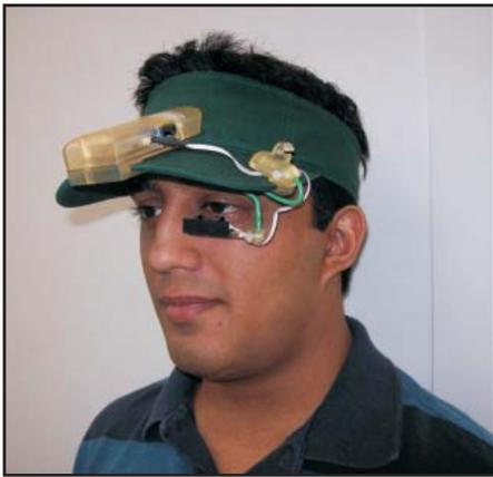
Figure 1. Subject wearing visor with attached head sensor (mounted on the visor) and eye sensor (positioned in front of the eye).
