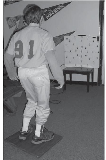
Figure 2. Subject on the Wayne Saccadic Fixator with balance board.
