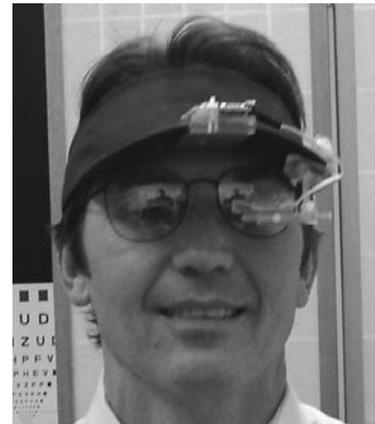
Figure 2. Subject wearing spectacle lenses and visor with attached head and eye sensors.
