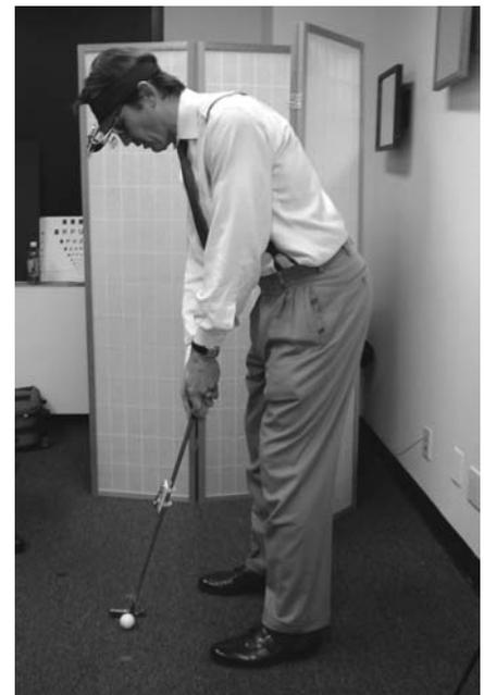
Figure 3. Subject putting while wearing recording system containing eye, head, and putting motion sensors.
