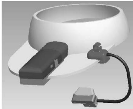
Figure 1. Visor with head sensor (attached to beak of visor) and eye sensor (below the visor).
