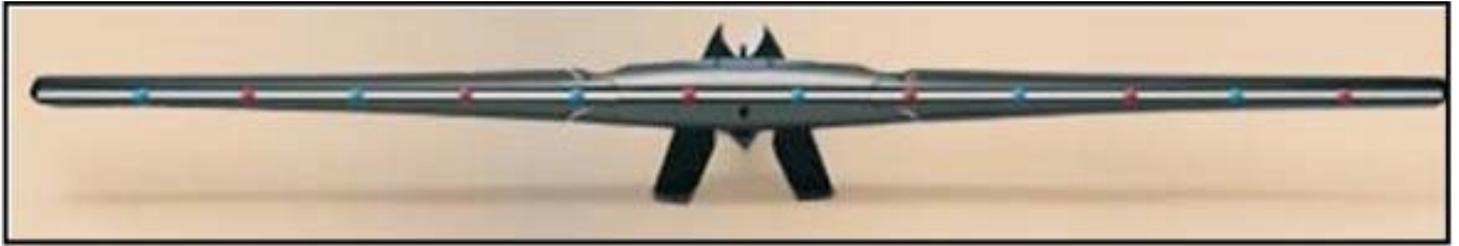
Figure 1. EYEPORTRM in the horizontal position, with the red and blue diodes visible.
