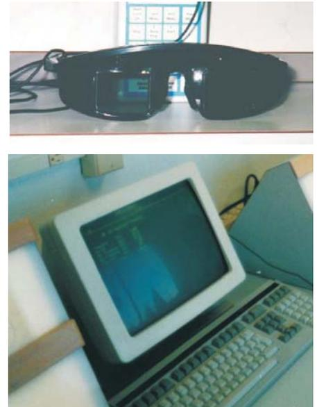
Figure 1. The prototype rapid alternate occlusion goggles (top picture) with control unit (bottom picture) used to set alternation rates.
